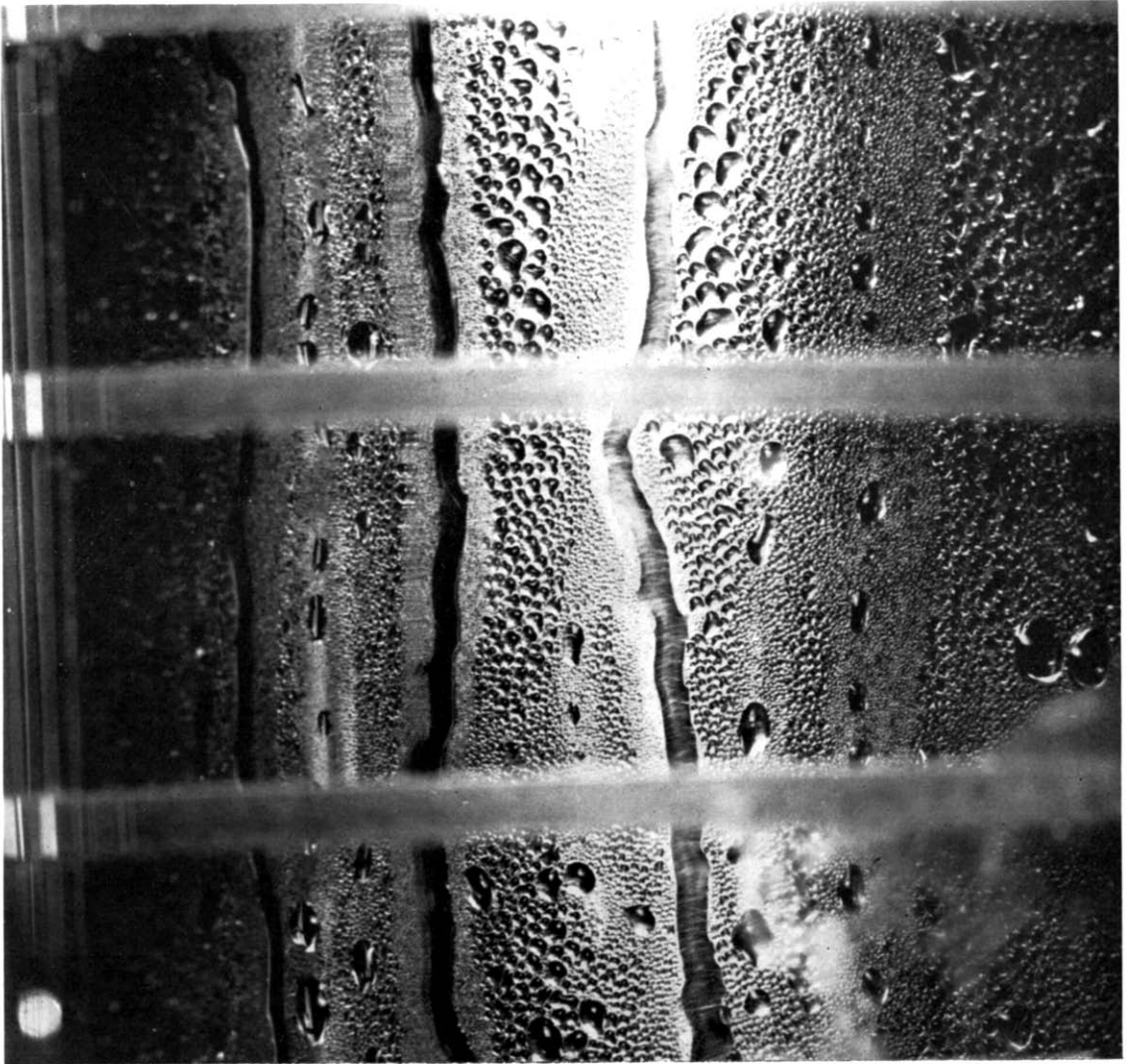
FIG. 2. Mixed dropwise and film condensation on a smooth chrome-plated surface (Ref. 21J).
